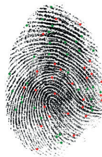
Image depicting an example of key minutiae feature points identified by an ievo control board
