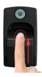
Place finger on sensor to activate (the sensor will illuminate).
